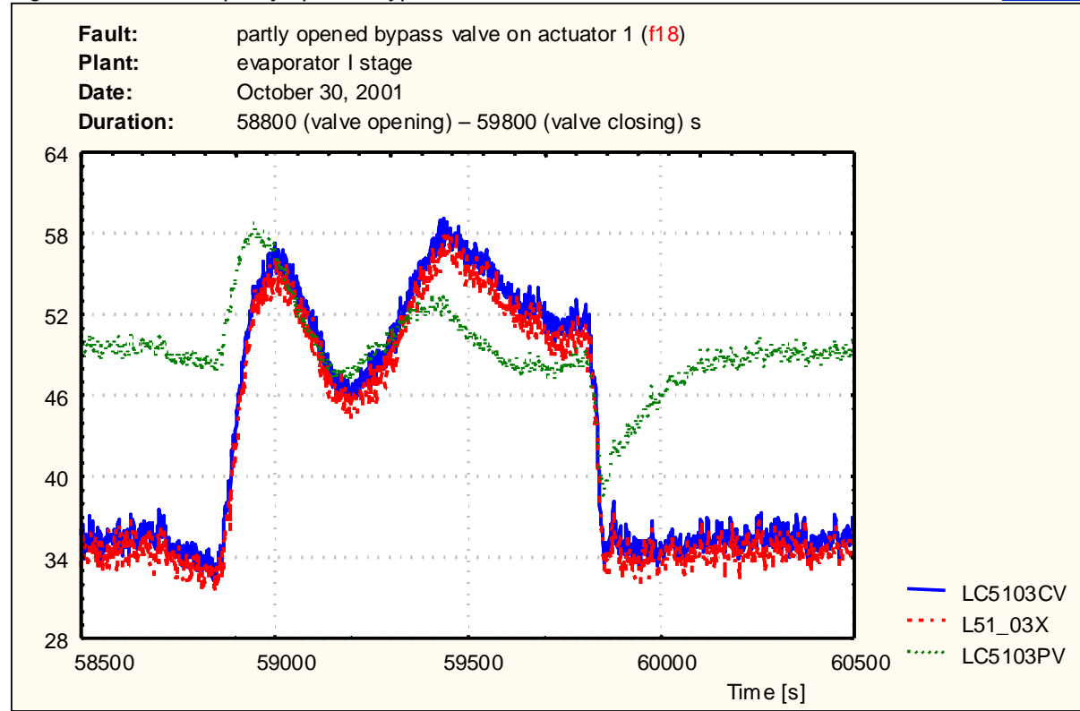
Figure 1. Fault f18 - partly opened bypass valve on Actuator 1
