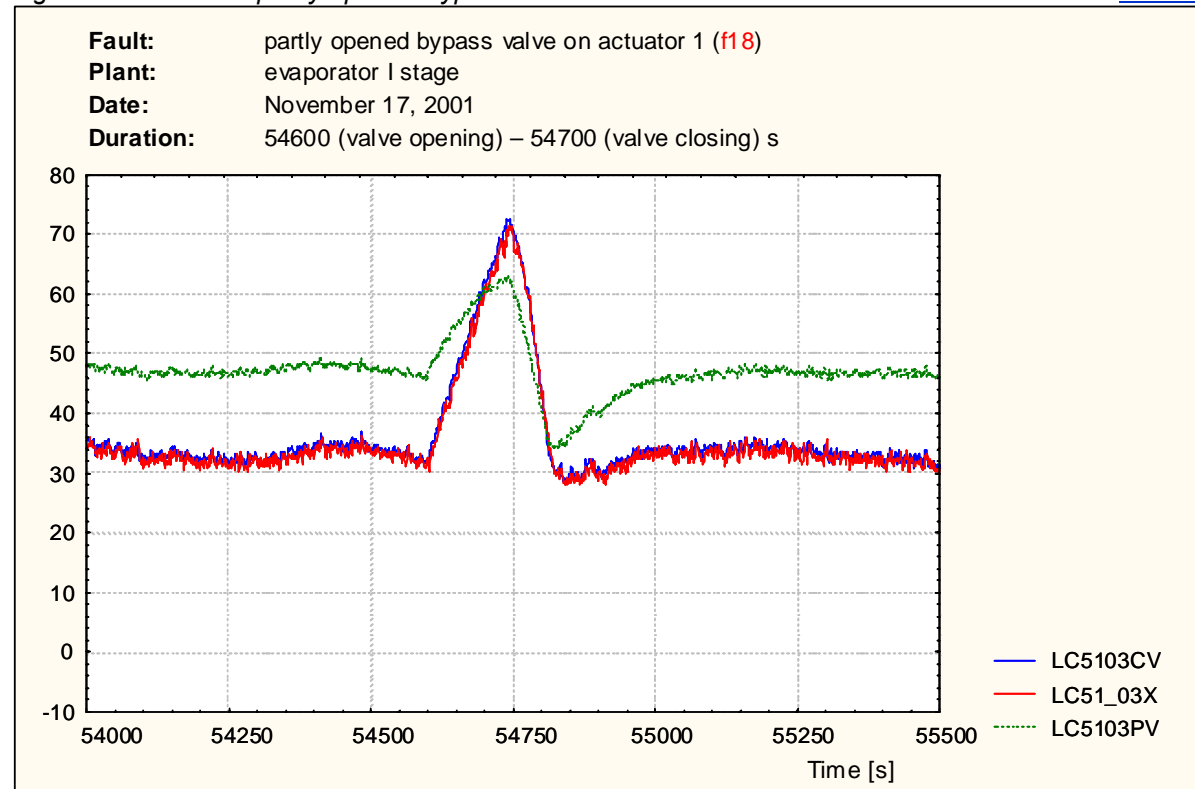
Figure 5. Fault f18 – partly opened bypass valve on Actuator 1
